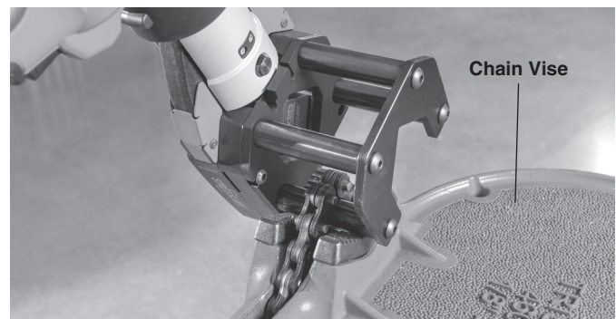
Figure 5 – Strut Shear Head Mounted in Chain Vise
