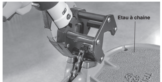
Figure 5 – Strut Shear Head Mounted in Chain Vise
