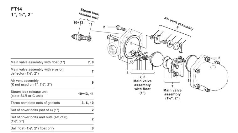
The erosion deflector on the 1" is pressed into the body during manufacture and not available as a spare.
