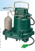
This model is constructed of the same heat-dissipating cast iron with powder coated epoxy finish, providing maximum pumping performance under the most extreme conditions. With Zoeller's cool run design, the hermetically-sealed, oil-filled motor and non-clogging vortex impeller add up to a long-lasting, trouble-free product. The heavy-duty power cord also includes an LED lighted plug.
