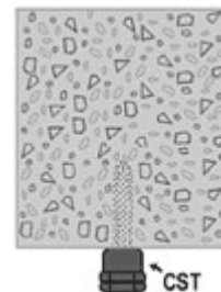
Use 20 ft/lbs torque on nut. For CST use 1/4" bit & drill 2" deep in concrete.
