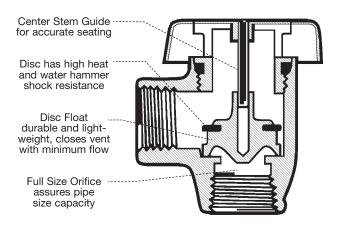
Since atmospheric type vacuum breakers are subject to normal maintenance and replacement, they should be located where emergency water spillage will create no problem and where they can be accessible for inspection or servicing.
