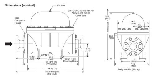
$^{\ast}$  The inlet connection on NPT and SW traps is a standard 4" (DN100) ANSI 300 RF Flange bolted to the trap body. The flange bore is 3" (DN80), NPT or SW to match the outlet connection of the trap.
