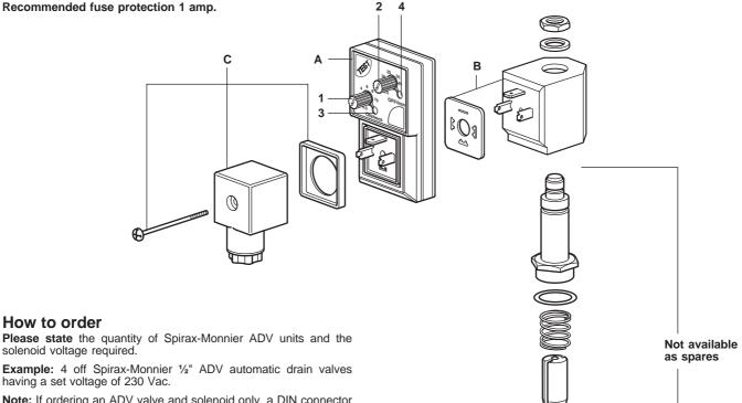
Note: If ordering an ADV valve and solenoid only, a DIN connector must also be ordered.
