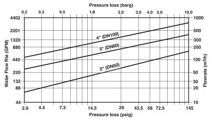
Pressure loss diagram with open valve at 68°F (20°C).
