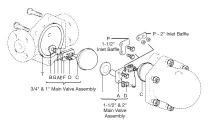
Valve Mechanism Kit w/ Float (3/4" & 1") A,B,C,D,E,F,G Valve Mechanism Kit (1-1/2" & 2") A,B,D,P Gasket Kit (3 sets of cover and Mechanism Gaskets) B,T
