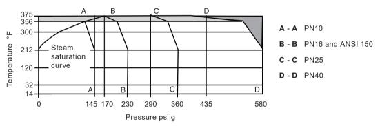
The product **must not** be used in this region or beyond the body design conditions quoted in the table below as damage to the internals will occur.
