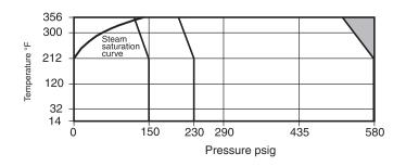
The product must not be used in this region or beyond the body design conditions quoted in the table below as damage to the internals will occur.
