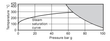
The product must not be used in this region or beyond the parameter of the PMA or TMA of the relative end connection.
