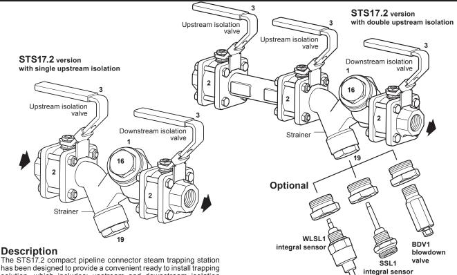
The STS17.2 compact pipeline connector steam trapping station has been designed to provide a convenient ready to install trapping solution, which includes: upstream and downstream isolation valves (2), body incorporating universal connector + strainer (1) and check valve blanking plug (16).
