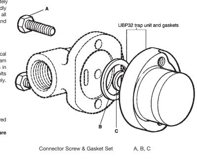
Available spare parts are shown in heavy outline. Parts drawn in broken line are not supplied as spares.
