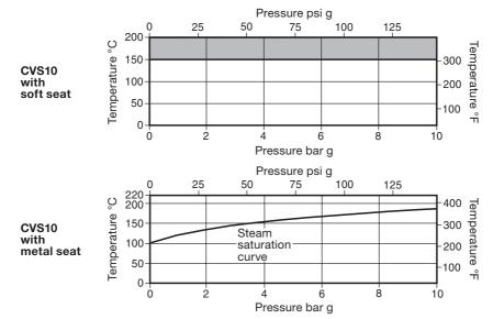
The CVS10 with EPDM seats must not be used in this region.
