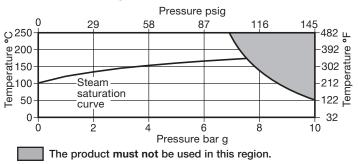
Note: For hygienic/sanitary clamp ends the maximum pressure / temperature may be restricted by the gasket or sanitary clamp used. Please consult Spirax Sarco.
