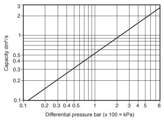
If the temperature of the air differs from 16°C, the discharge capacity from the graph can be corrected by miltiplying it by the following equation: 289
