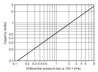
If the temperature of the air differs from 16 °C, the discharge capacity from the graph can be corrected by multiplying it by the following equation:
