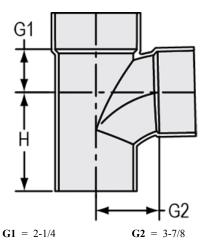
**Type** Sanitary Tee Street **Connection** Spig x Hub x Hub
