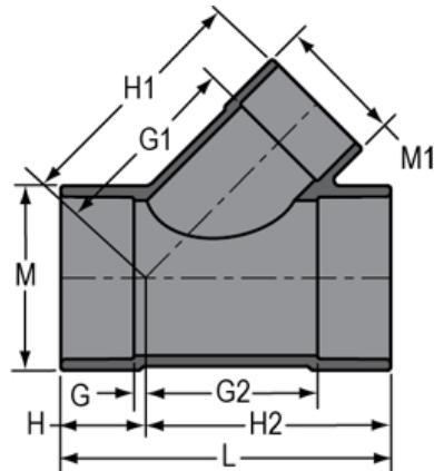
**Connection** Socket x Socket x Socket
