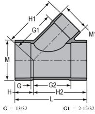
**Connection** Socket x Socket x Socket
