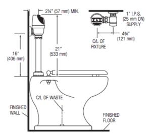
When installing the G2 Optima Plus in a handicap stall: Per the ADA Guidelines (section 604.9.4) it is recommended that the grab bars be split or shifted to the wide side of the stall. If grab bars must be present over the valve, use the Alternate ADA Installation as shown to the right.
