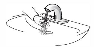
Place hands under faucet. Solenoid valve should "click," LED in sensor window should blink once and water should flow from the spout.
