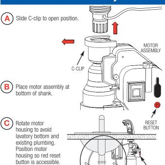
Push the motor assembly up into place and secure by pushing the C-clip closed.
