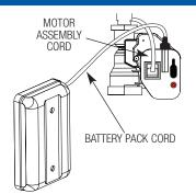
Connect the power cord from the battery pack by inserting then screwing clockwise into inlet on top of motor assembly.
