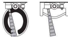
3. When the user steps away from the Object Lock Infrared Sensor, the circuit initiates the flushing cycle to flush the fixture. The Circuit then automatically resets and is ready for the next user.
