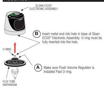
Push Diaphragm securely against underside of Sloan ECOS® Electronic Assembly. Place entire Assembly onto the Valve Body.
