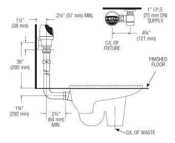
Model 8115 & 8116 valves are designed for installations where the water supply is roughed-in 24" - 27" (610 mm - 686 mm) above the top of the water closet.
