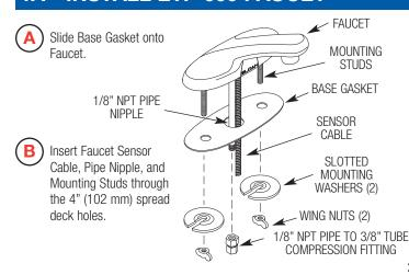
Secure Faucet to deck using Slotted Mounting Washers and Wing Nuts supplied.
