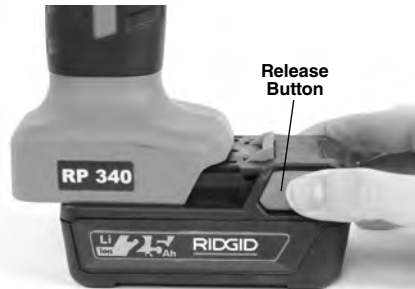
Figure 11 – Installing/Removing Battery In Tool
