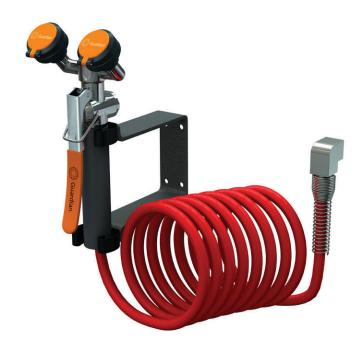
**Application:** Dual purpose eyewash/drench hose with 12' coiled hose for wall mounting. Unit meets the provisions of ANSI Z358.1-2014 as both an eyewash and a drench hose. Unit may be left in the mounting bracket for use as a fixed eyewash, leaving user's hands free. Alternatively, unit may be removed for use as a drench hose to rinse any part of user's eyes, face or body. 12' nylon retractable hose coils to eliminate trip hazard.
