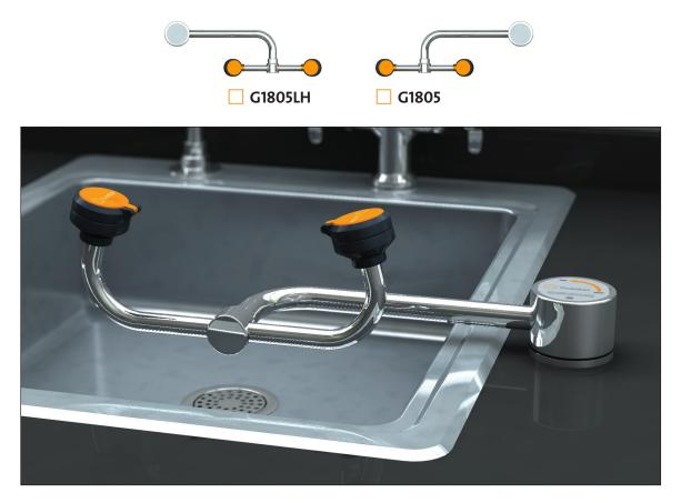
**Application:** AutoFlow<sup>™</sup> eyewash for mounting next to sink. Swinging the spray head assembly horizontally out over the sink activates the water flow. The unit remains in operation until the spray head assembly is swung back into the storage position, closing the valve.
