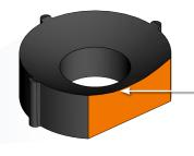
**IMPORTANT** In order to operate properly, the flow control must be inserted into the body concave end first.
