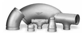
Gruvlok Series Stainless Steel Fittings are full flow design with ends grooved to Gruvlok specifications. The Series standard material is formed from Type 304 Stainless Steel. The Series Fittings are annealed after forming and grooving to provide increased corrosion resistance. Gruvlok Series Stainless Steel 45° and 90° elbows and tees have compact center-to-end dimensions which make installation quick and easy with the Gruvlok Figure 7400SS Coupling, or other Gruvlok products.
