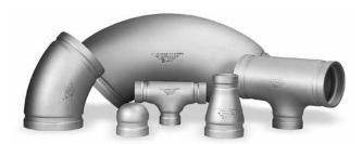
Gruvlok Series Stainless Steel Fittings are full flow design with ends grooved to Gruvlok specifications. The Series standard material is formed from Type 304 Stainless Steel. The Series Fittings are annealed after forming and grooving to provide increased corrosion resistance. Gruvlok Series Stainless Steel 45° and 90° elbows and tees have compact center-to-end dimensions which make installation quick and easy with the Gruvlok Figure 7400SS Coupling, or other Gruvlok products.
