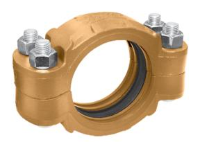
Gruvlok Fig. 7377 is a flexible coupling utilizing double groove technology designed for high pressure piping applications. Fig. 7377 is specifically designed for use in mining, oil, gas, slurry, sludge, and hydraulic systems. The maximum working pressure for each pipe schedule and size are listed in the table below. Fig. 7377 is an ideal solution for high pressure applications, exceeding Anvil's Fig. 7004 capabilities. See page 3 for double groove piping dimensions.
