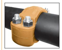
**FINAL ASSEMBLY**— Visually inspect the pipe joint to ensure the coupling keys are fully engaged in the pipe grooves, both bolt pads are a firm and even metel-to-metal contact, and the gasket is not visible.
