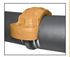
HOUSINGS— Place each half of the coupling housing over the gasket, making sure the housing keys engage the pipe grooves.
