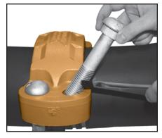
**BOLTS**— Apply a thin coat of Xtreme Lube to the bolt threads. Tighten the nuts alternately and equally to the specified bolt torque.
