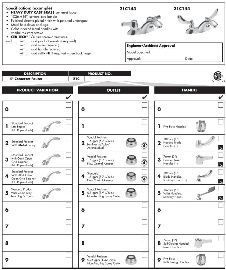
See Series 27C4, 27C5 for 4" Gooseneck Spout Centersets. (1) H & C Temperature Indicator available. Add suffix -TI. Refer to www.specselect.com for individual models. Flow Rates are at 60 PSI. Note: Use this page front and back as a product submittal sheet.
