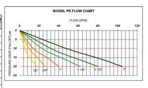
Note: Flow curves are based on static conditions of 100psi inlet pressure and 50 psi outlet pressure.
