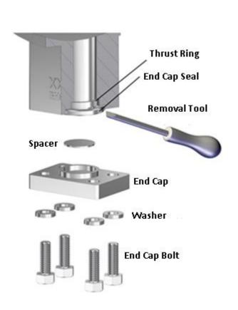
FIGURE 9. END CAP SEAL REPLACEMENT
