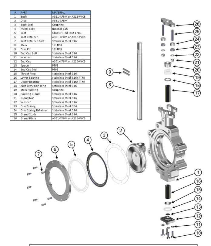
FIGURE 11. FIRE SAFE SEATED EXPLODED VIEW
