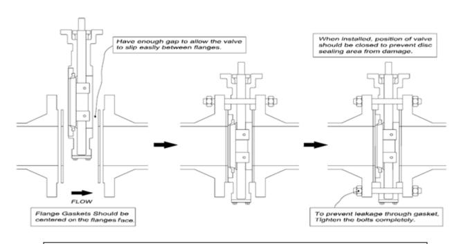
**FIGURE 3. INSTALLATION DIAGRAM**
