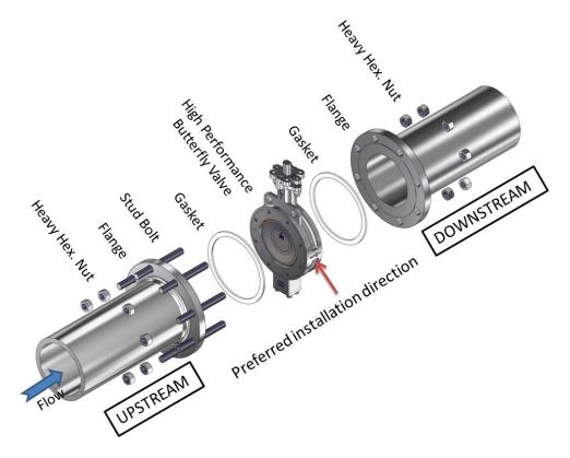
Preferred installation direction is flow into the disc's face. See arrow on side of valve for preferred flow direction.
