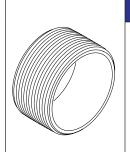
Butt Nipples are intended for joining couplings or female threaded components end to end without exposing male threads. Butt Nipples have standard NPT male threads on both ends. Threads may have fewer imperfect threads due to reduced nipple length. Butt Nipples are fabricated from ASTM A53 Schedule 40 welded pipe.
