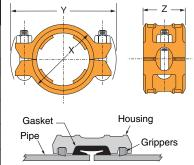
Working pressure and end load are based on a properly assembled Roughneck coupling with bolts fully torqued to the above specifications, on plain-end or beveled standard wall steel pipe and Gruvlok Plain- End Fittings.
