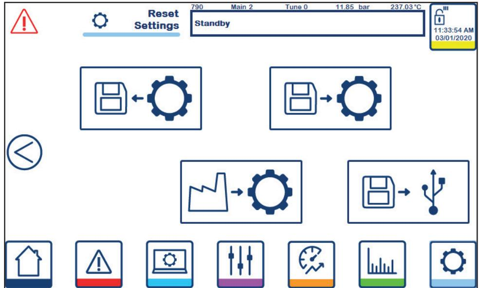
Factory reset (790) allows users to save, load and reset the current settings and configuration of the CSG-HS. (only available in standby mode)
