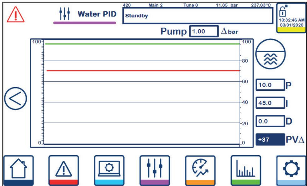
Water PID settings (420) also includes the pump offset value and a live PID graph showing the process and control values, and the process set-point.
