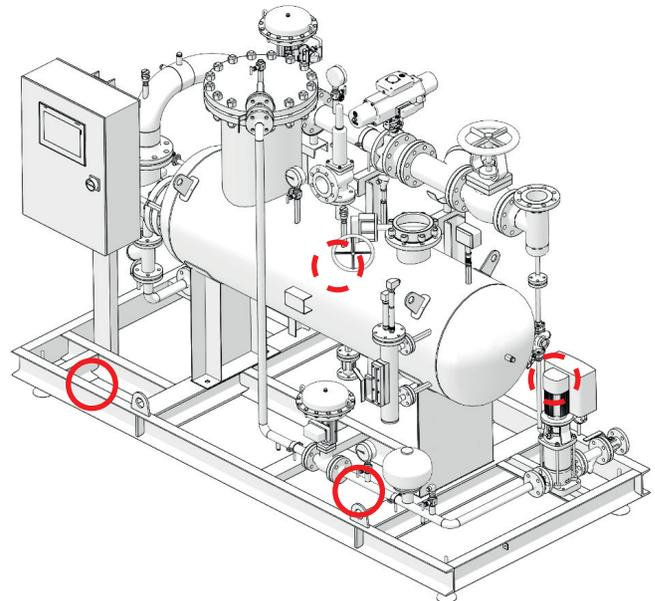
Ring-nut for extraction/withdrawal of mounting foot
