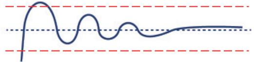
If the process value continues to exceed the band tolerances and the timer continues past the Band Alarm time, then a Control Band Alarm is issued to the Alarms screen. If the process value returns to within the band tolerances, the timer is reset. Control Bands only monitor in Run mode and not in the PID Tuning sequence. Alarms and Alerts reset when the process value returns to within the upper and lower bands.
