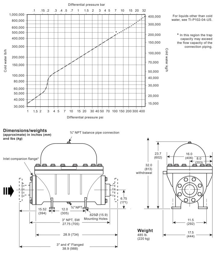
\* The inlet connection on NPT and SW traps is a standard 4" (DN100) ANSI 300 RF Flange bolted to the trap body. The flange bore is 3" (DN80), NPT or SW to match the outlet connection of the trap.
